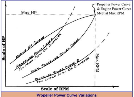
the output power that your engine can deliver. What the propeller power curve shows is *approximately* the power that a standard propeller would be using at any given engine RPM. You can see just how different the shape between the two curves is—between the BHP (or SHP) curve and the propeller curve.
