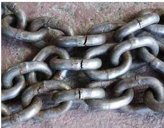
Stainless Anchor Chain Failure At Welds
