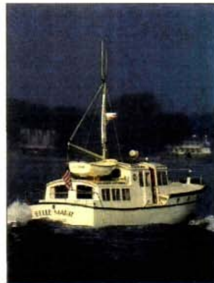
Pushed by a well-protected propeller and able to float in 19" of water, BELLE MARIE can cruise just about wherever she chooses. PETITE BELLE, a 9'6" Nutshell pram, rides comfortably on the housetop.
