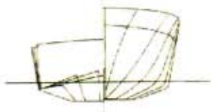
The hull's bottom, a full 2 1/2" of plywood sheathed with 60-oz biaxial E-glass and epoxy, can take the ground without problems.
